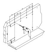
**CAUTION!** Check the wall condition and make sure the selected wall plugs can support the full weight of the radiator filled with the heating medium. Technical specifications of the radiator can be found on the last page of this manual and on the website: www.termaheat.pl.
