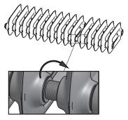
8. Determine how deep the collar turning key needs to go and mark this distance on the key shaft with e.g. a thick marker (see image below).
