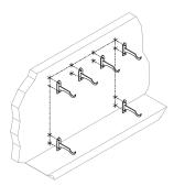
13. While hanging the radiator use the included straps. If this is a free-standing model, use the straps while moving it to the installation location.
