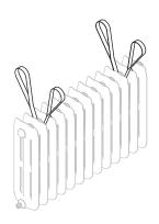
4. Special caution must be taken while lifting up the radiator from the pallet.
